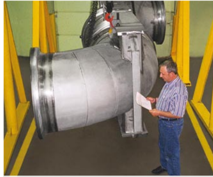
Figure 2. A 42 in. diameter TC guide spool designed and manufactured by PHPK.
