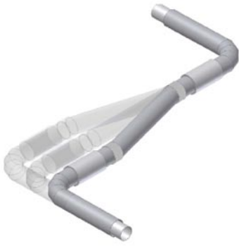
Figure 1. Movement modelled for a vacuum insulated thermal compensation guide (TC guide).
