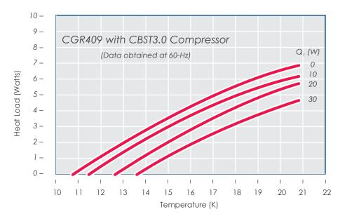
(Second stage refrigeration capacity as a function of first stage heat load)
